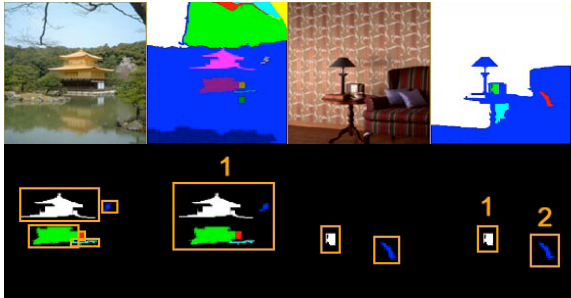
Figure 3. Extracting features: System retrieves feature areas through image segmentation (top). If the distance between regions is less than the threshold, regions are merged as a new region (bottom).
