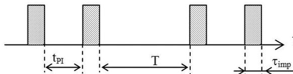
Figure 1. The time diagram of sequence of pair light impulses
