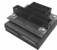
Figure 8. Sensor controller with housing and custom connection board
