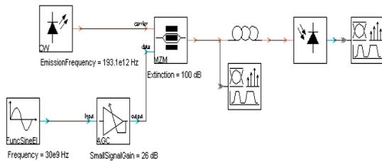
Figure 8. VPI scheme for setup, depicted on Fig. 7
