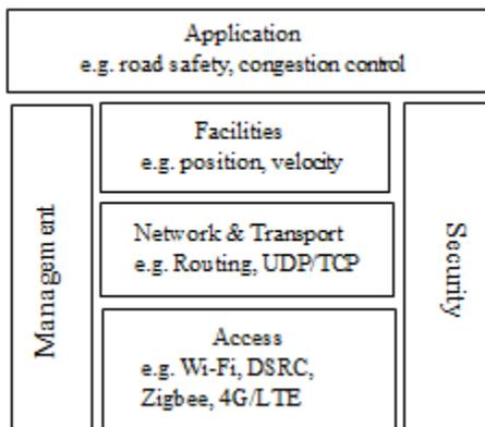
Figure 2. ITS reference traffic structure (adapted from [16])
