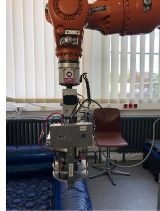
Figure 1b. Sensors mounted on the miniature drill-head and further mounted on the KUKA robotic arm
