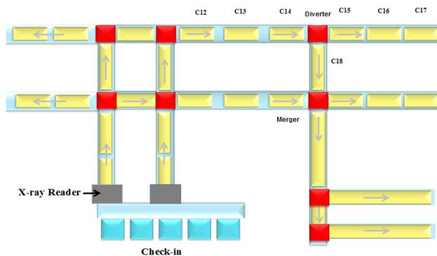
Figure 8. The baggage handling system structure.
