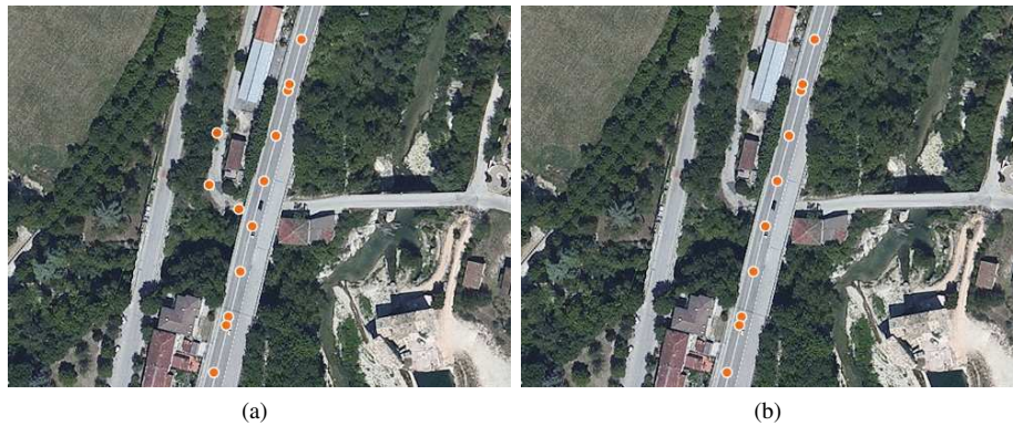
Figure 4. Projected trace points plotted on top of the satellite map showing examples of Case-2: (a) before and (b) after match enhancement.
