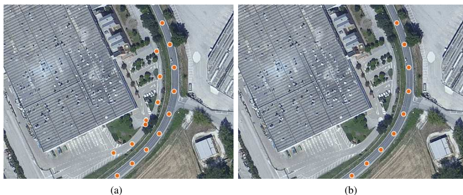
Figure 7. Projected trace points plotted on top of the satellite map showing examples of Case-4: (a) before and (b) after match enhancement.
