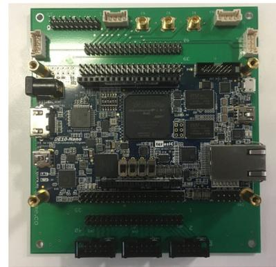
Figure 9. Signal processing board.
