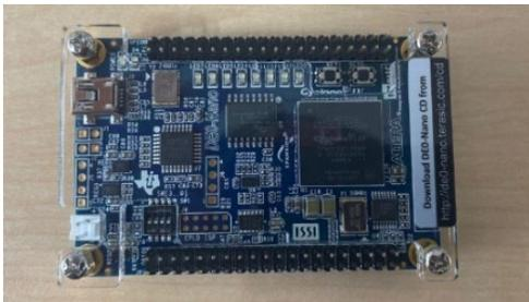
Figure 20. FPGA for LED control.
