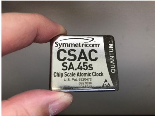
Figure 1. Chip Scale Atomic Clock (CSAC).
