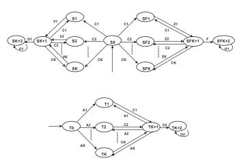
Fig. 2: A system with two components  $G_1$  (top) and  $G_2$  (bottom) for proving undecidability of joint diagnosability.
