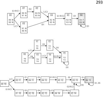
Fig. 7: Part of the renamed local twin plant for  $G_1$  (top), part of renamed local twin checker for  $G_2$  (middle) and part of the left consistent plant  $T_f^l$  (bottom).
