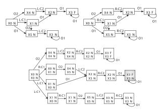
Fig. 4: Two instances of the diagnoser for  $G_1$  (top) and part of the corresponding local twin plant (bottom).
