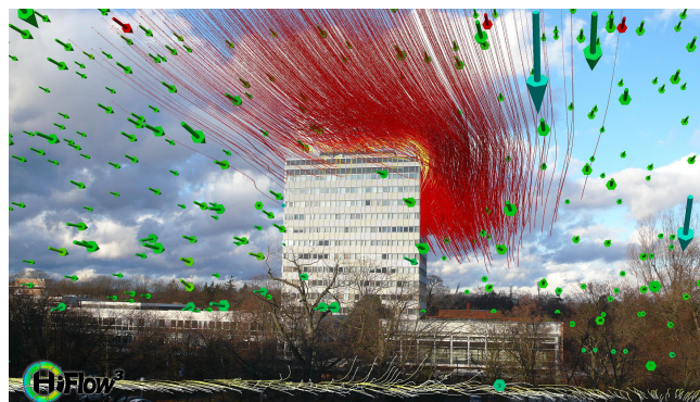
Figure 18. Augmented Reality visualization of velocity field and distributed fine dust particles around the Physics buildings, created using the masking technique.
