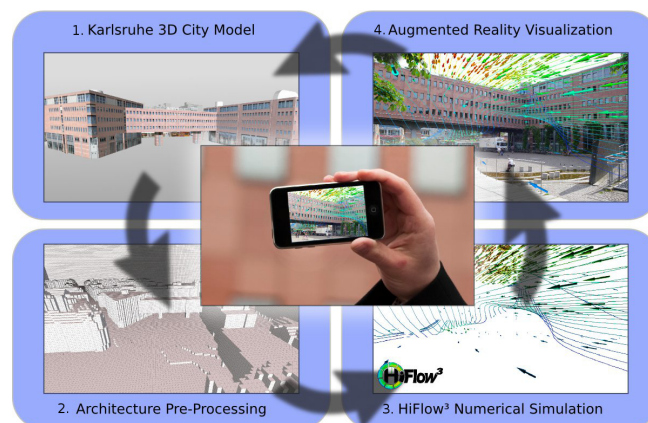
Figure 1. Augmented Reality simulation and visualization workflow.
