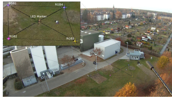
Figure 9. Marker detection from UAV camera view.
