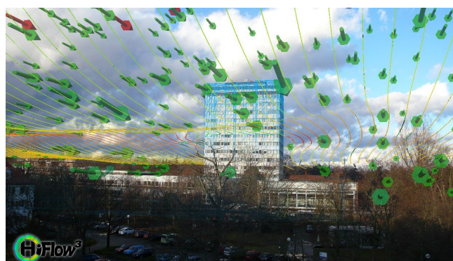
Figure 17. Augmented Reality visualization of air flow around isolated building from the Physics scenario.
