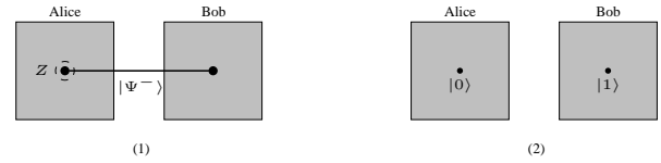
Fig. 5. Illustration of the BBM protocol [5]. Here, Alice performs a measurement in the Z -basis.
