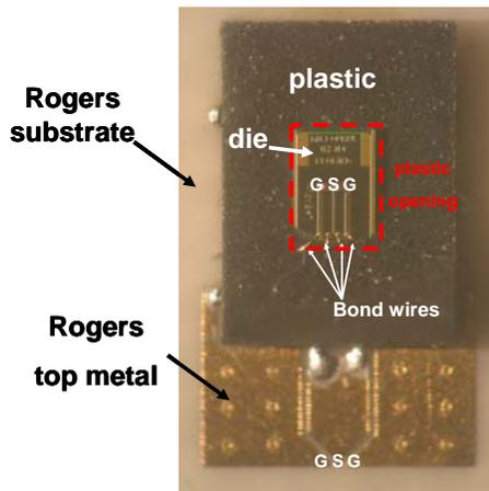
Figure 9. Photograph of the designed test-case suitable for microwave package characterization and modeling. Configuration allows 2 ports micro-probing: one on the inner die and the second one on the Rogers top metal (bottom of the picture)
