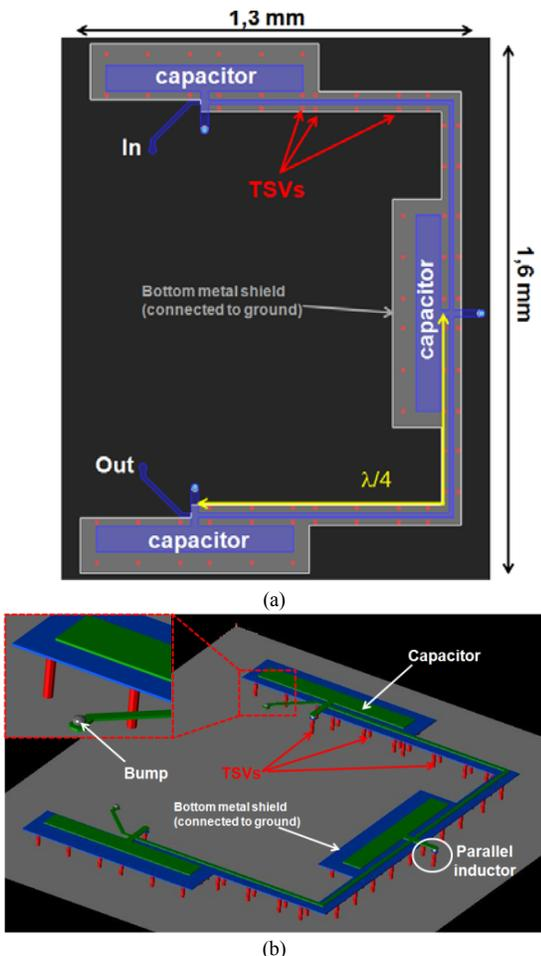
Figure 20. Top view (a) and 3D view – the gray bottom plate is the ground reference of the device (b) of the simulated band-pass filter
