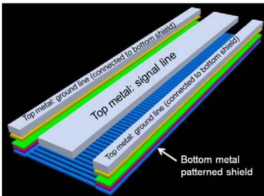
Figure 15. Layout pattern of the considered transmission lines used to calibrate the 3D EM simulator
