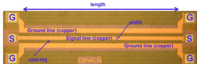
Figure 16. Photograph of a transmission line within GSG pads for two-ports S-parameter measurements, used to calibrate the 3D EM simulator
