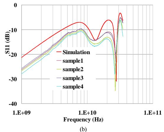
Figure 10. Comparison between measurements and simulated data vs. frequency on the package test-case – (a) transmission parameter, (b) reflection parameter
