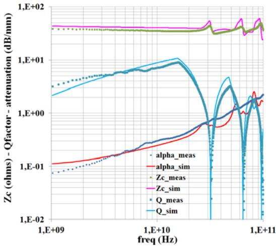
Figure 18. Comparison between measured and simulated data vs. frequency for transmission line characteristic impedance  $Z_c$ , attenuation alpha and quality factor Q (length = 2000  $\mu\text{m}$ , width = 15  $\mu\text{m}$ , spacing = 8.3  $\mu\text{m}$ )
