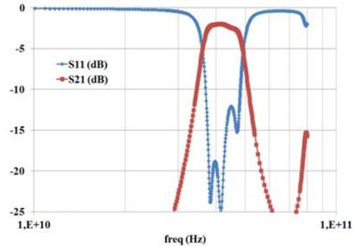
Figure 21. Simulated variations of transmission and reflection S-parameter of the proposed filter (nominal process parameters with copper back-end)
