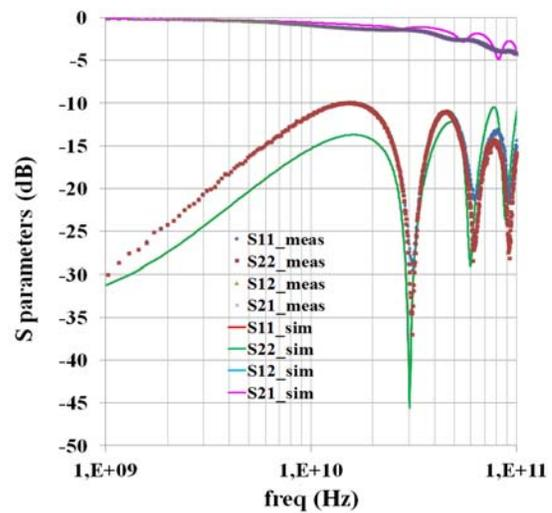
Figure 17. Comparison between simulated (EM) and measured S-parameter obtained on a transmission line (length = 2000  $\mu\text{m}$ , width = 15  $\mu\text{m}$ , spacing = 8.3  $\mu\text{m}$ )
