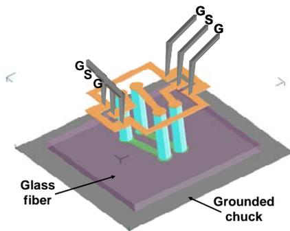
Figure 4. Illustration of the measurement test-bench used to guarantee a good ground reference together with an isolation between bottom metal traces and chuck (case of a 2-turns solenoid)
