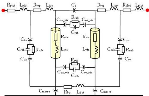
Figure 5. Schematic view of the equivalent circuit consider to derive the compact electrical model of 3D TSV based solenoid
