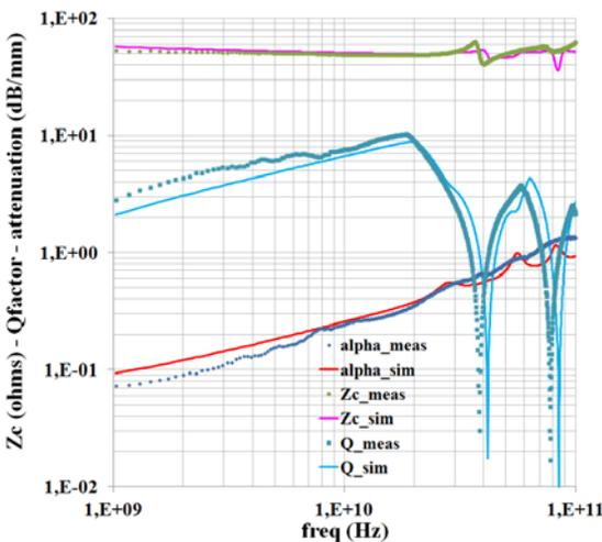
Figure 19. Comparison between measured and simulated data vs. frequency for transmission line characteristic impedance  $Z_c$ , attenuation alpha and quality factor Q (length = 2000  $\mu\text{m}$ , width = 15  $\mu\text{m}$ , spacing = 8.3  $\mu\text{m}$ , 4 bends)
