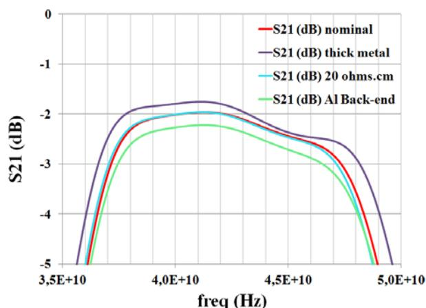
Figure 22. Variations of the Insertion Loss vs. frequency for different process options
