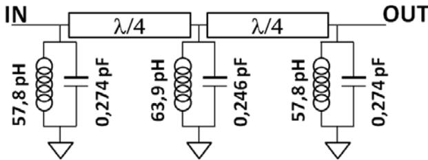
Figure 14. Schematic view of the 3<sup>rd</sup> order 42 GHz band-pass filter considered
