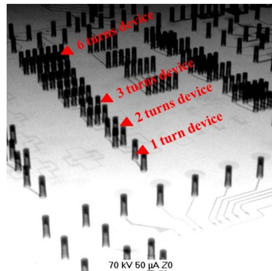
Figure 3. X-ray diffraction picture of the solenoid dedicated module (source IPDiA) – The bottom white face of the picture is the top side of the wafer
