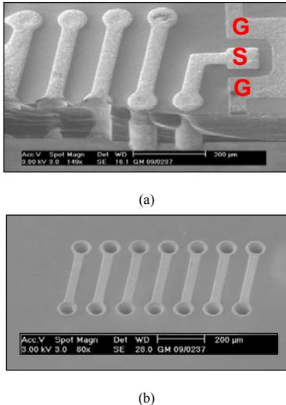
Figure 1. SEM pictures Top view (a) and bottom view (b) of the 3D solenoids within GSG (Ground Signal Ground) pads – source IPDiA
