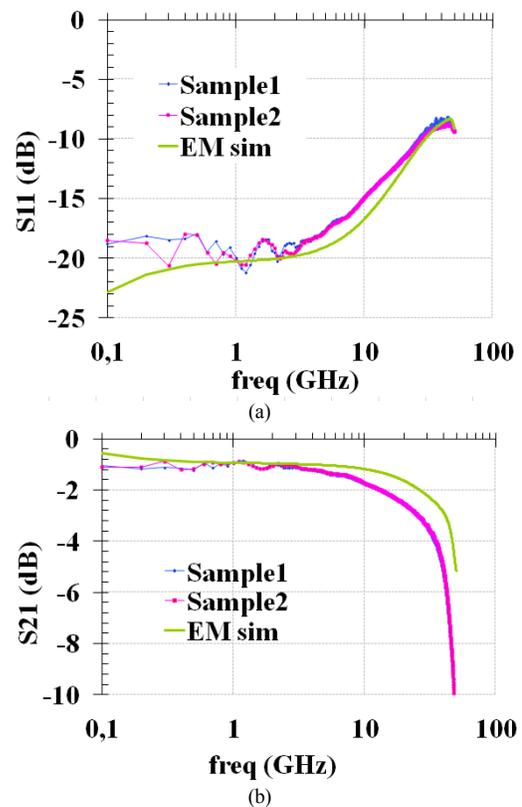
Figure 7. Comparison between Measured and simulated data on both (a) Reflection and (b) transmission S-parameter (1-turn solenoid)
