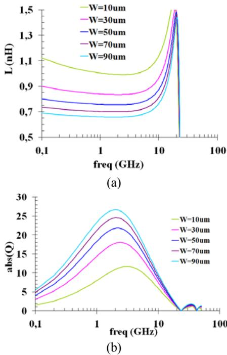
Figure 6. Simulated variations of (a) the self-inductance value and (b) quality factor vs. frequency for 1-turn solenoid ( $D_y$  was set to a fixed value during the simulations). These plots have been deduced from 2-ports S-parameter analysis with a classical CAD simulator (i.e., SPICE). Compact model described in the previous paragraph has been used to extract the devices performances
