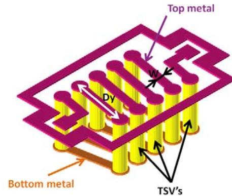
Figure 2. Synoptic representation of a 5 turns 3D solenoid within its RF test structure (bulk silicon is not represented on the picture)
