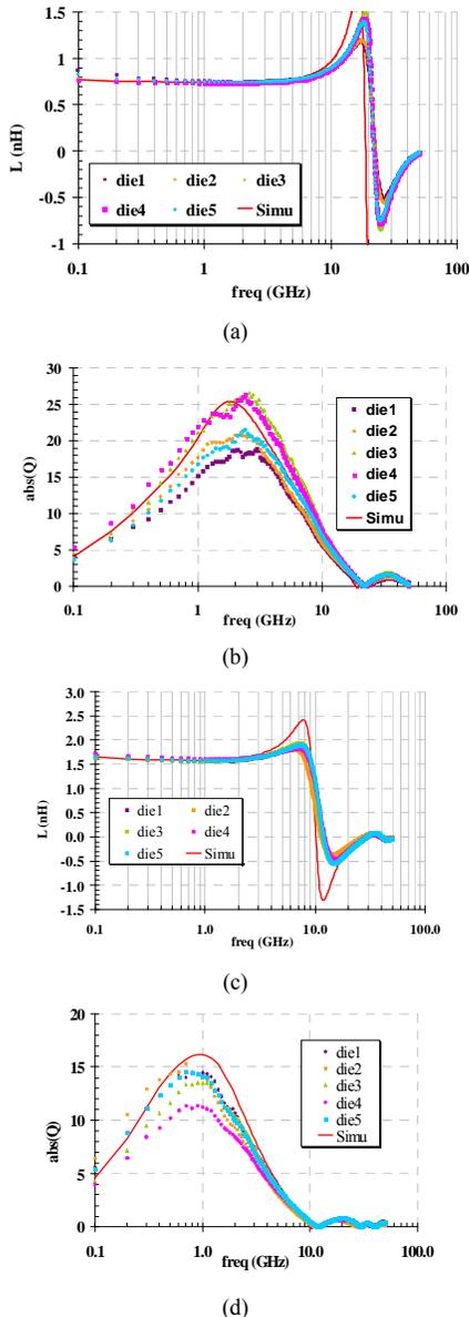
Figure 8. Comparison between measured and simulated data for 1-turn solenoid (a): self-inductance value (b) quality factor and 2-turns solenoid (c): self-inductance value (d) quality factor
