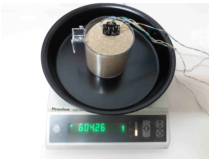
Figure 7. Sensor calibration with Tottori sand.
