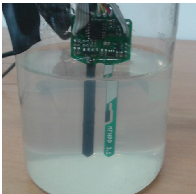
Figure 6. Probe distance calibration in agar solution
