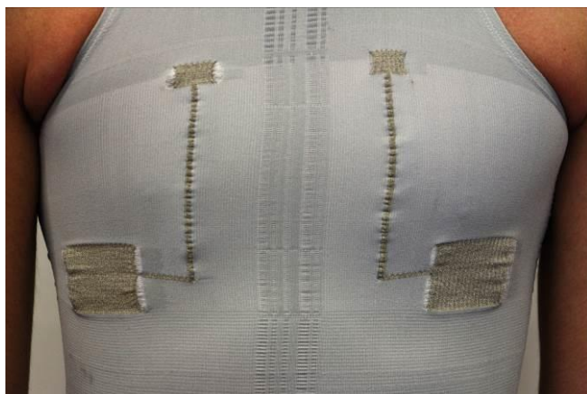
Figure 7. Shirt front view with ECG electrodes.
