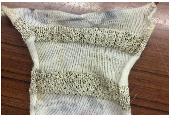
Figure 12. Sample for preliminary moisture sensor test.
