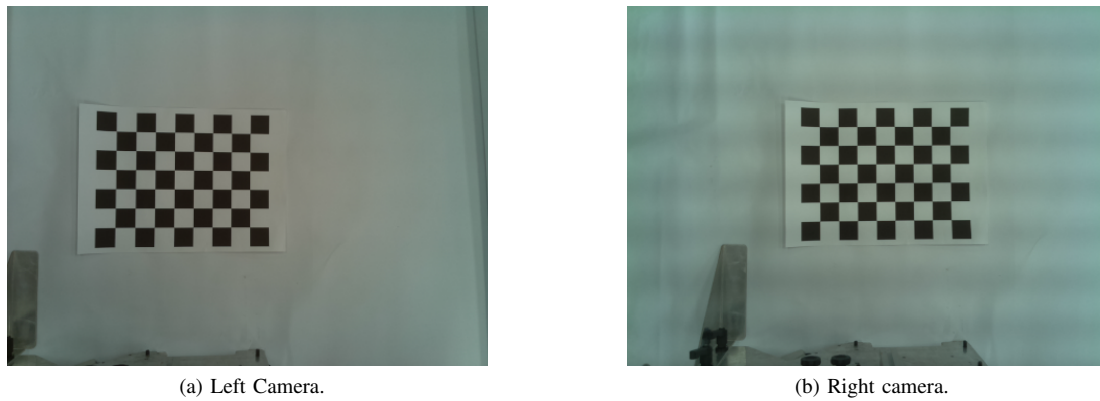
Figure 7. Images of a calibration chessboard, captured synchronously and without being processed.
