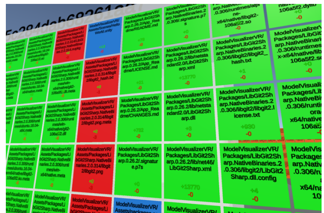
Figure 22. Commit files added (green), changed (blue), deleted (red); number of lines affected indicated in each tile at the bottom.
