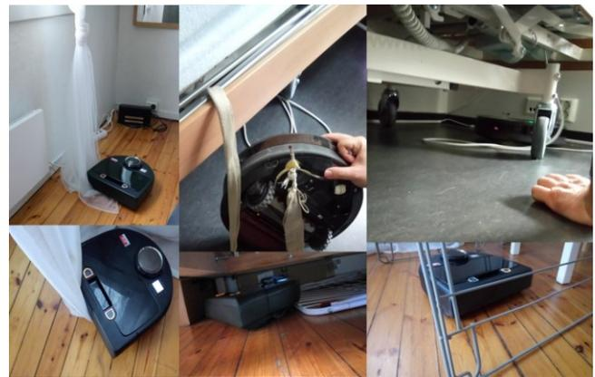
Figure 6. Situations where the robot got stuck and needed facilitation work
