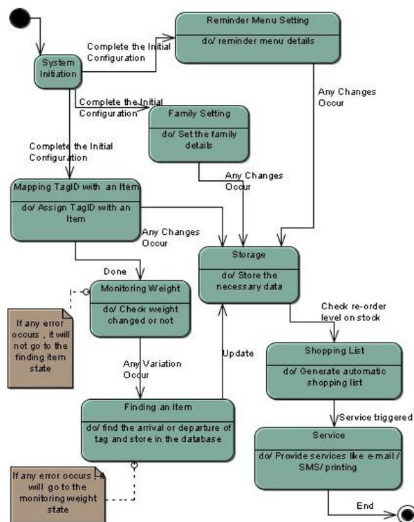
Figure 3. State Transition diagram of Smart Kitchen Cabinet
