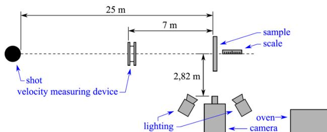
Figure 3. Experimental set-up.
