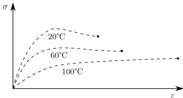
Figure 2. Qualitative effects of the temperature on the stress-strain-diagram of thermoplastics with decreasing fail-stress  $\sigma_f$  and increasing fail-strain  $\epsilon_f$  at higher temperatures.
