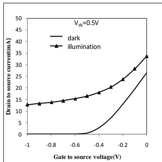
Figure 3. Variation of drain current with gate to source voltage under illumination and dark condition for a 100 nm InAlAs/InGaAs HEMT. ( $\lambda=0.623$  um and  $P_{op}=10$  Watt/cm<sup>2</sup>).
