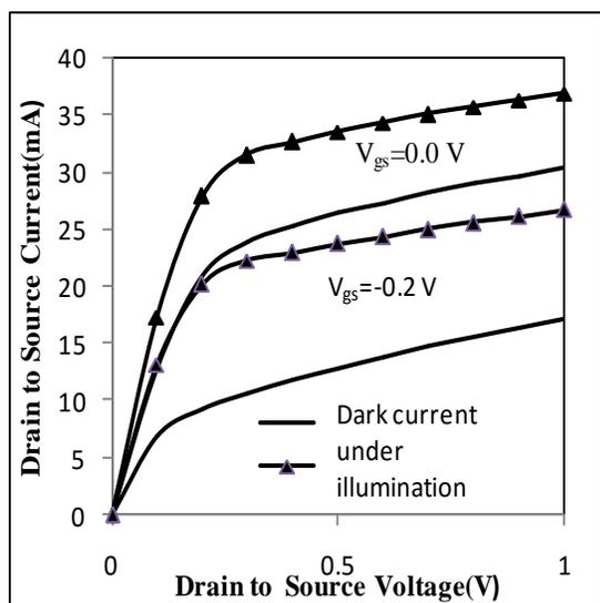
Figure 2. Variation of drain to source current with drain to source voltage under illumination and dark condition for a 100 nm InAlAs/InGaAs HEMT ( $\lambda=0.623$  um and  $P_{op}=10$  Watt/cm<sup>2</sup>).
