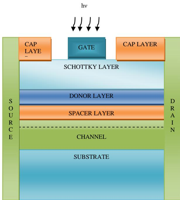
Figure 1. Simulated structure of InAlAs/InGaAs HEMT under illumination.
