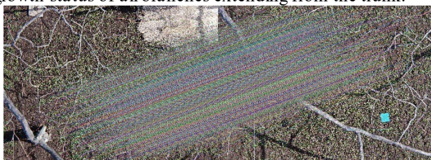
Figure 3. Feature Point Pairs from Two Overlapping Aerial Photographs
