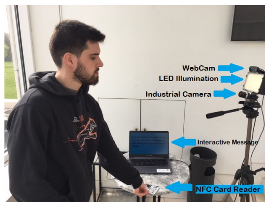
Figure 7. Set up of the system for the experimental results.
