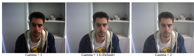
Figure 5. Images acquired with gamma of 1, 1.6 and 2 respectively.
