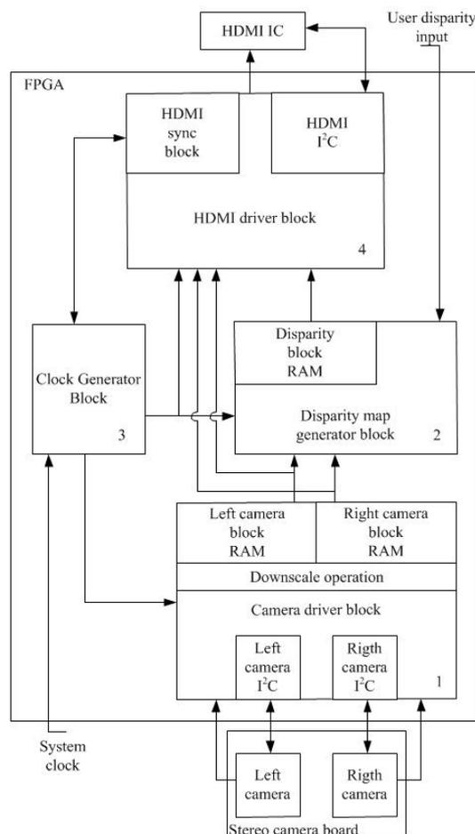
Figure 2. General Structure of hardware
