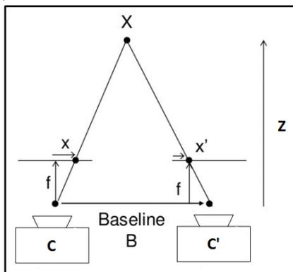
Figure 1. The relation between disparity ( $x-x'$ ), baseline ( $B$ ), focal length ( $f$ ) and the distance ( $Z$ ) between camera and the object “X”
