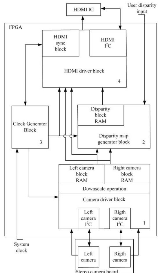
Figure 2. General Structure of hardware
