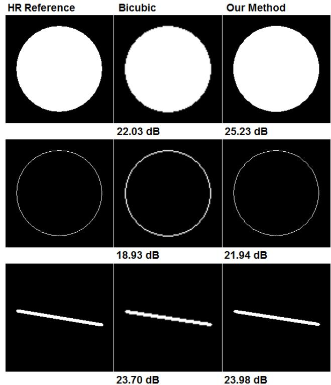
Figure 7. PSNR comparison of Bicubic interpolation and our method.
