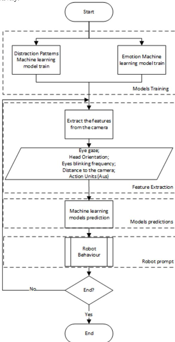
Figure 2. System flowchart highlighting the defined modules for detecting distraction patterns and emotional states: Models training, Feature extraction, Models predictions, and Robot prompt.
