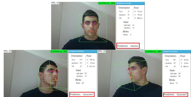
Figure 5. The GUI displaying the classification considering different poses (results using Gaussian SVM method). The classifier output is presented in the interface (red rectangles).
