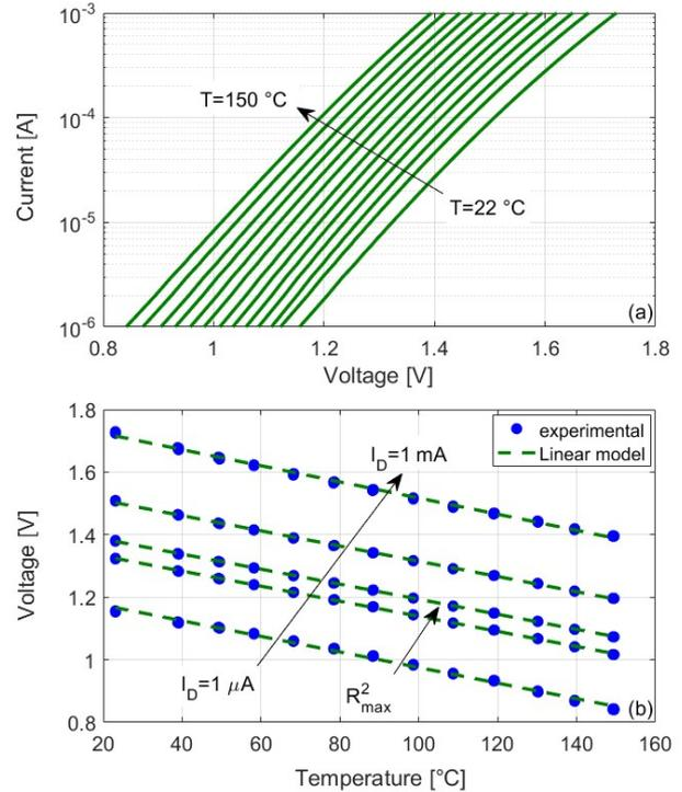
Figure 3. (a) Current-voltage ( $I_D-V_{BD}$ ) characteristics in the temperature range  $T=22-150^\circ\text{C}$  in steps of 10  $^\circ\text{C}$ . (b) Measured (points) body-drain voltage versus temperature. Experimental data are fitted with the best-calculated linear model.
