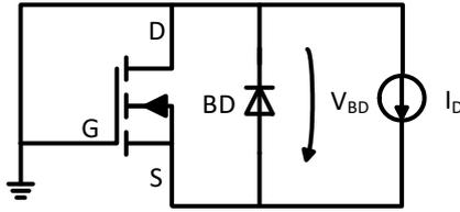
Figure 1. Electrical circuit for the measurement of the body-drain voltage ( $V_{BD}$ ) in the bias current range from 1  $\mu\text{A}$  up to 1 mA.
