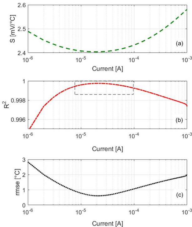
Figure 4. (a) Sensitivity,  $S$ ; (b) coefficient of determination,  $R^2$ ; and (c) root mean square error,  $rmse$ , within the whole temperature range of 22-150 °C and for bias currents in the range  $I_D=1 \mu\text{A}$ -1 mA.
