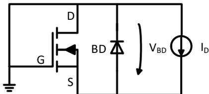
Figure 1. Electrical circuit for the measurement of the body-drain voltage ( $V_{BD}$ ) in the bias current range from 1  $\mu\text{A}$  up to 1 mA.
