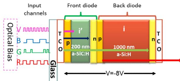
Figure 4. Double pi-n/pin configuration and device operation.
