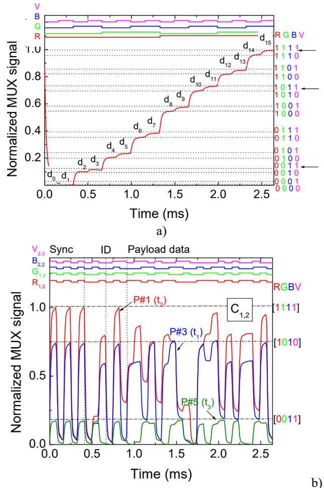
Figure 5. MUX/DEMUX signals under 390 nm front irradiation. On the top the transmitted channels packets [R, G, B, V] are decoded. a) Calibration cell. b) MUX signal in three successive instants ( $t_1, t_2, t_3$ ).
