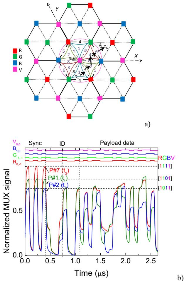
Figure 6. a) Fine-grained indoor localization and navigation, as illustrated by the arrows. b) Signal acquisition at  $t_1$ ,  $t_2$  and  $t_3$ . On the top the transmitted channels packets [R, G, B, V] are decoded
