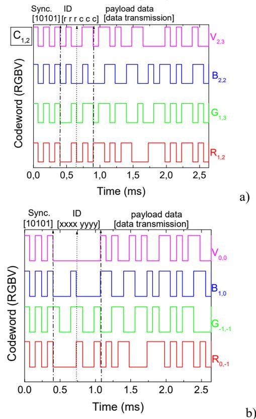
Figure 3. Frame structure. Representation of one original encoded message, in a time slot. a) Square topology;  $R_{12}$ ;  $G_{1,3}$ ;  $B_{2,2}$  and  $V_{2,3}$  are the transmitted node packet from the  $C_{1,2}$  array in the network.. b) Hexagonal topology;  $R_{0,-1}$ ;  $G_{-1,-1}$ ;  $B_{1,0}$  and  $V_{0,0}$  are the transmitted node packet of the unit cell in the network.
