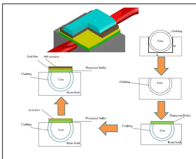
Figure 1. SPR sensor platform based on D-shaped POF.
