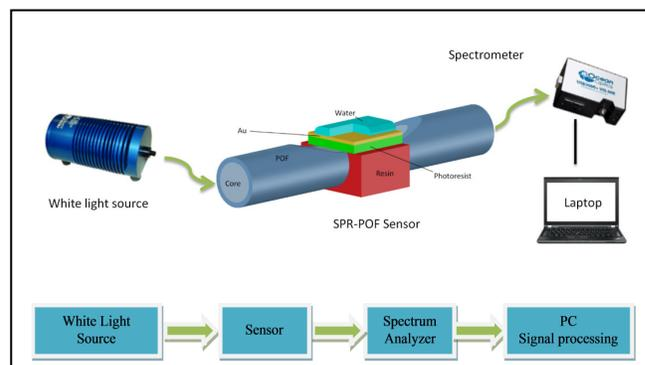
Figure 2. Experimental setup.
