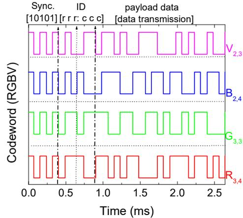
Figure 4. Frame structure. Representation of one original encoded message [10101][rrr ccc: XY...].  $R_{3,4}$ ,  $G_{3,3}$ ,  $B_{2,4}$  and  $V_{2,3}$  are the transmitted node packet, in a time slot, from the crossroad in the network.
