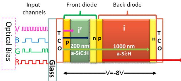
Figure 5. Double pin configuration and device operation.
