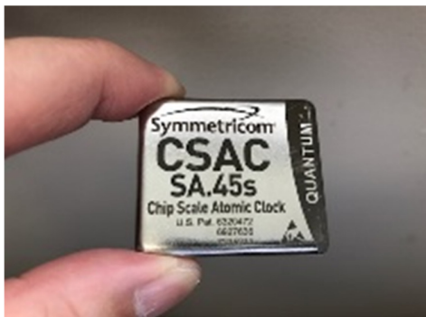
Figure 1. Chip Scale Atomic Clock (CSAC).
