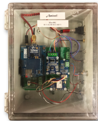
Figure 6. Example of developed radio module enclosure or sensor node.
