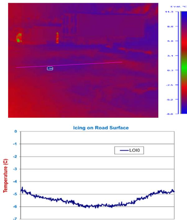
Figure 3. Surface temperature distribution along iced road surface.
