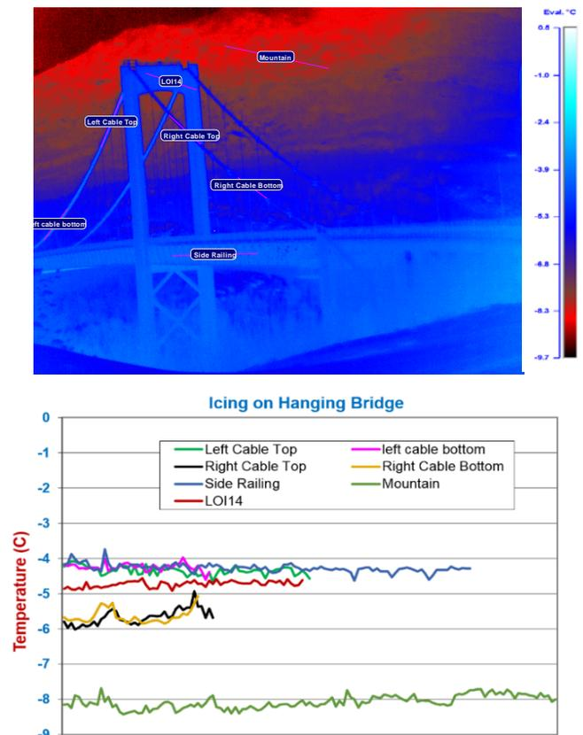
Figure 2. Surface temperature distribution along different sections of iced bridge
