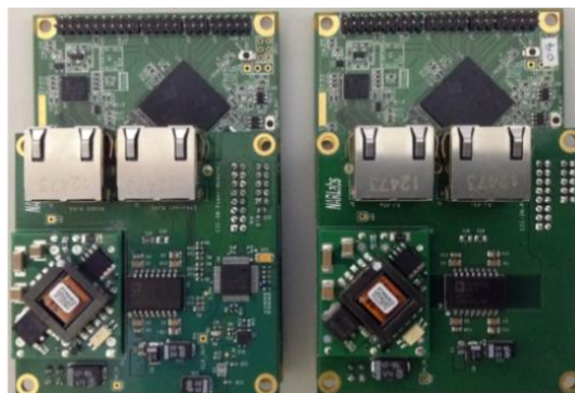
Figure 4. The pictures of printed circuit boards of gateway (left) and sensor node (right).
