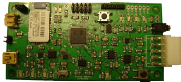
Figure 9. ECG subsystem printed circuit board.
