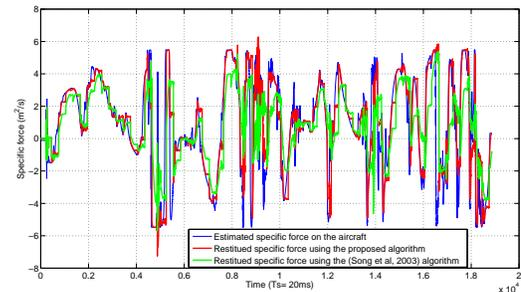
Fig. 8: Restituted specific force using the [19] algorithm vs restituted specific force using the proposed algorithm.
