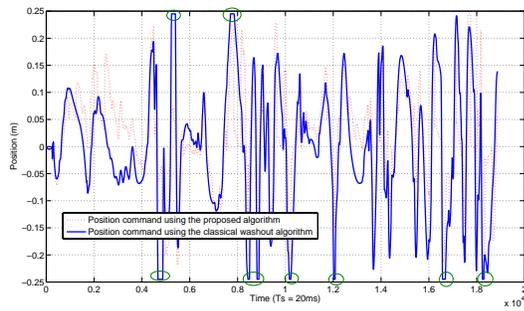
Fig. 9: Comparison of the position commands using the classical washout algorithm vs restituted the position commands using the proposed algorithm.
