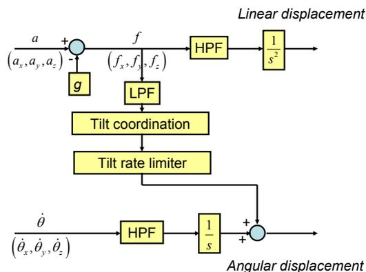
Fig. 1: Classical washout filter flowchart.
