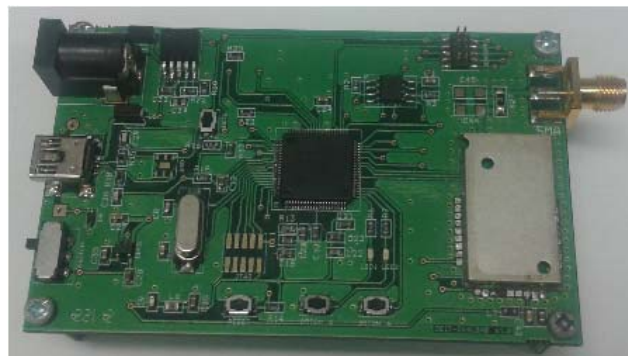
Fig. 5 Picture of the developed wireless M-BUS Gateway
