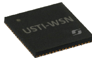
Figure 6. USTI-WSN IC prototype in 64-pad QFN package.
