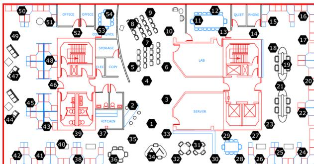
Figure 1. Sensor deployment in Intel Berkeley lab dataset.
