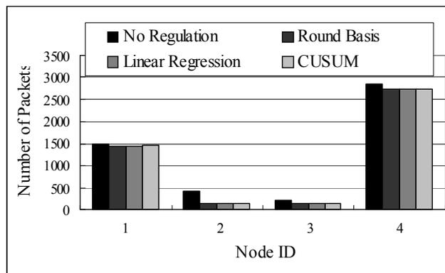
Figure 4. Number of network packets transmitted by nodes 1-4.
