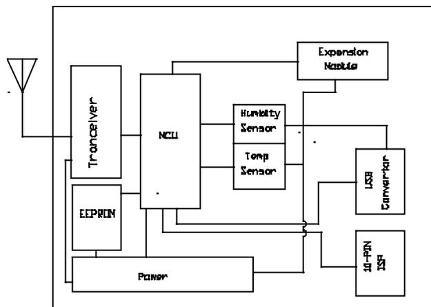
Figure 3. Detailed Block Diagram of the Sensor Node.
