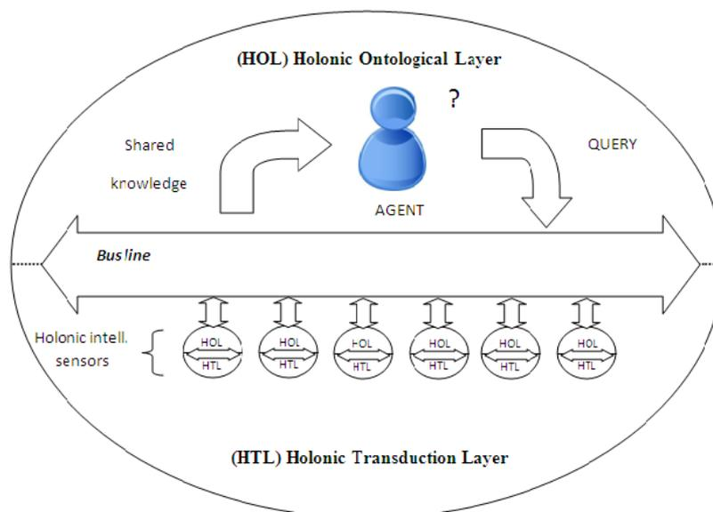
Figure 3. Conceptual model of a holonic intelligent sensor-based system. Since the model is recursive, the image accounts for a generic granular representation level.
