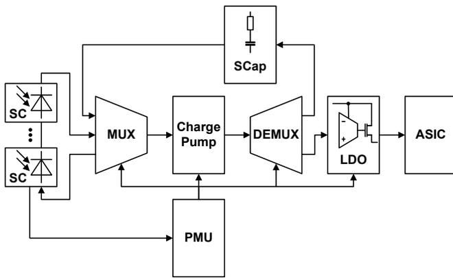
Fig. 7. Power Supply Sensor Node.
