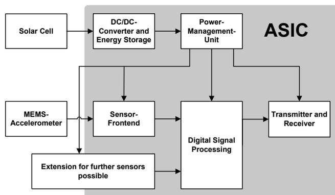
Fig. 6. Block diagram sensor node.
