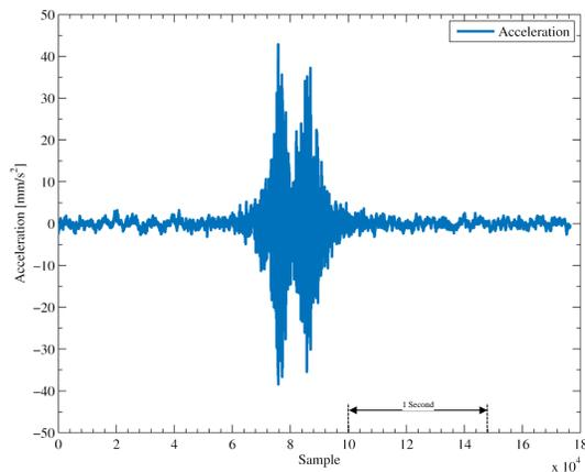
Fig. 3. Passing car with 50 km/h in 30 cm distance.
