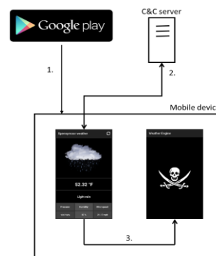
Figure 3. Mechanism of bot dissemination employed by Spennymoor Weather
