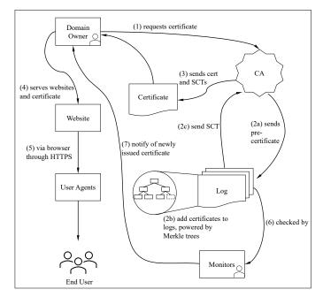
Fig. 3. Implementation of certification transparency (illustration based on [19]).
