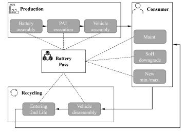
Fig. 4. Battery pass as life cycle record.
