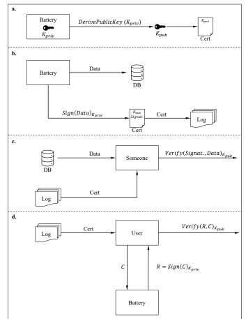
Fig. 5. Implementation of digital pass with certificates. **a.** Enrollment phase **b.** Update of battery records **c.** Verify that the certificate belongs to records **d.** Verify that the battery belongs to the certificate.
