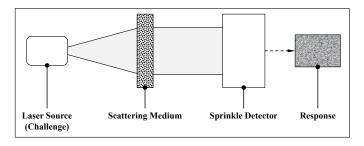
Fig. 1. Process of optical PUF (illustration based on [16])
