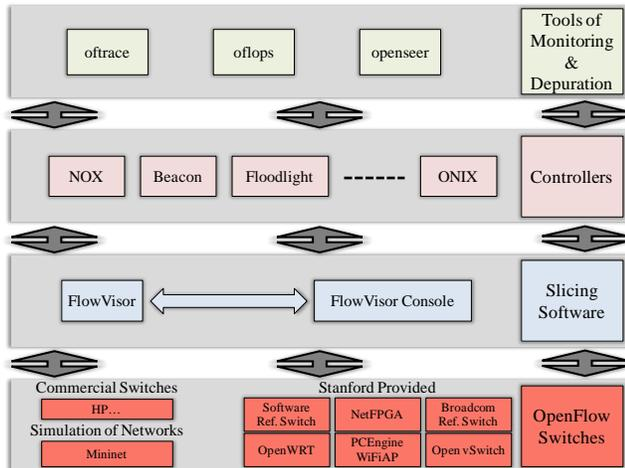
Figure 1. Key component of SDN in layered structure.
