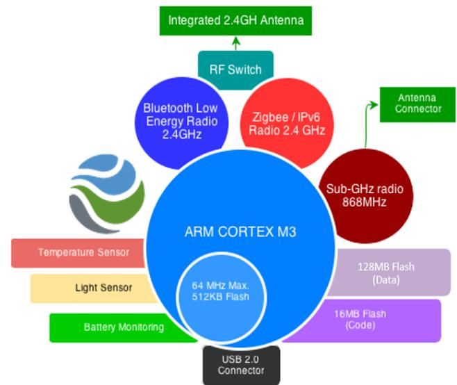
Figure 3. Block diagram of AUTHENTIC Platform functionality.
