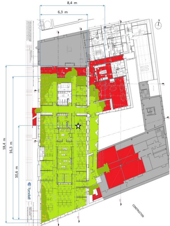
Figure 10. ZigBee 2.4GHz range test
