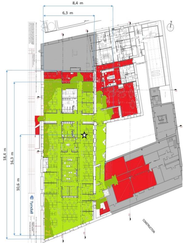
Figure 10. ZigBee 2.4GHz range test
