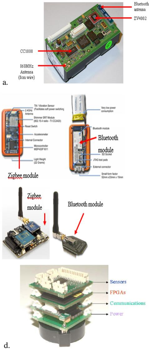
Figure 1. Multiradio systems. a) Dual Radio BTnodeRev3 b) Dual Radio Shimmer c) Wasp Mote ZigBee & Bluetooth Modules d) The Tyndall 25mm modular system
