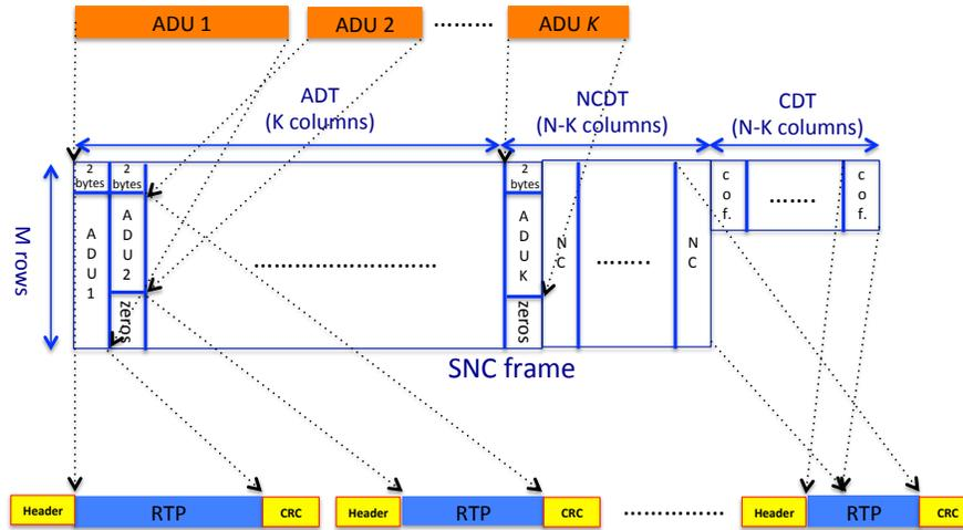
Figure. 3: Encapsulation of application layer data units over RTP with network coding.
