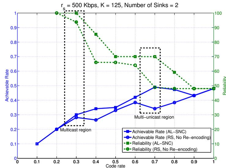
(b) AL-SNC multicast and multi-unicast regions with video codec rate  $r_s = 500$  Kbps.
