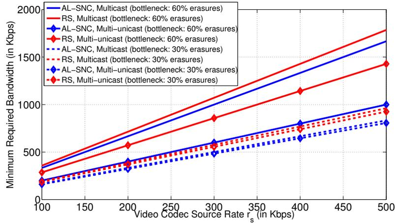
Figure. 8: Minimum network bandwidth requirement for multicast and multi-unicast with AL-SNC.
