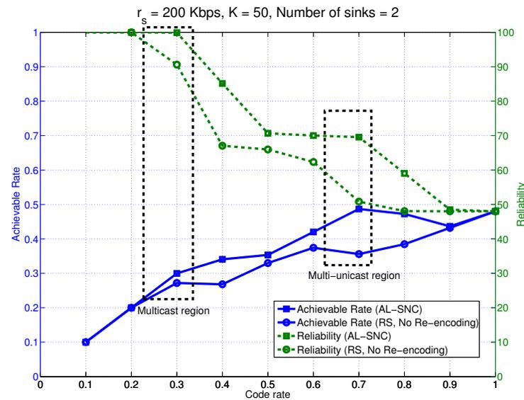
(a) AL-SNC multicast and multi-unicast regions with video codec rate  $r_s = 200$  Kbps.
