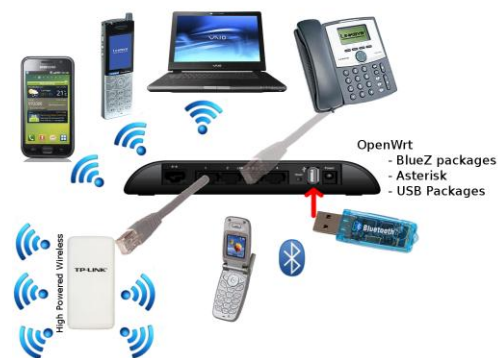
Figure 7. Proposed wireless expansion of OpenWrt based Blue Bridge.
