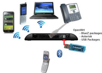
Figure 4. Proposed OpenWrt infrastructure for low cost community telephone network.
