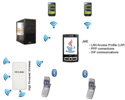
Figure 8. Proposed wireless expansion of cell phone based Blue Bridge.
