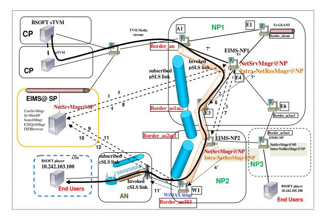
Figure 9. UPB testbed infrastructure: installation of pSLS link and cSLS link in NP1, NP2 and in WiMAX Access Network.
