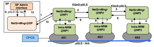
Figure 2. Basic pSLS invocation chain of signalling (3 IP domains).
