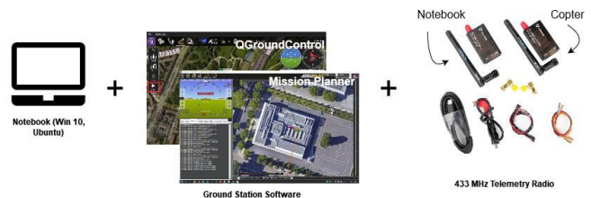
Figure 5. Ground Station system architecture.
